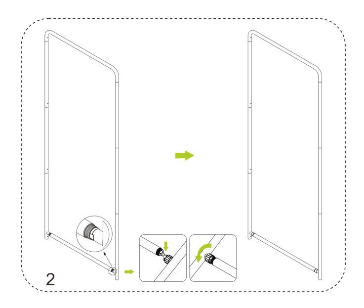
2. Using the big plastic screw parts to fasten the bottom cross bar
