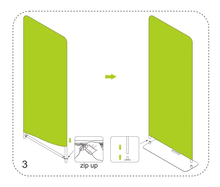
3. To wrap the fabric banner on the frame and zip up, afterwards install whole display stand to the base.
