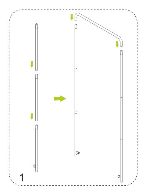
1. To connect all the aluminium tubes according to the numbering
